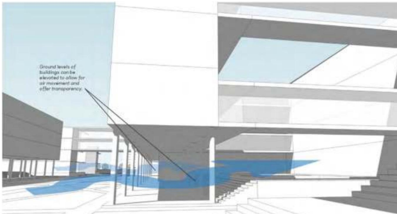
In addition to providing shaded walkways, the elevated area also allows for continuous air circulation in the courtyard.
