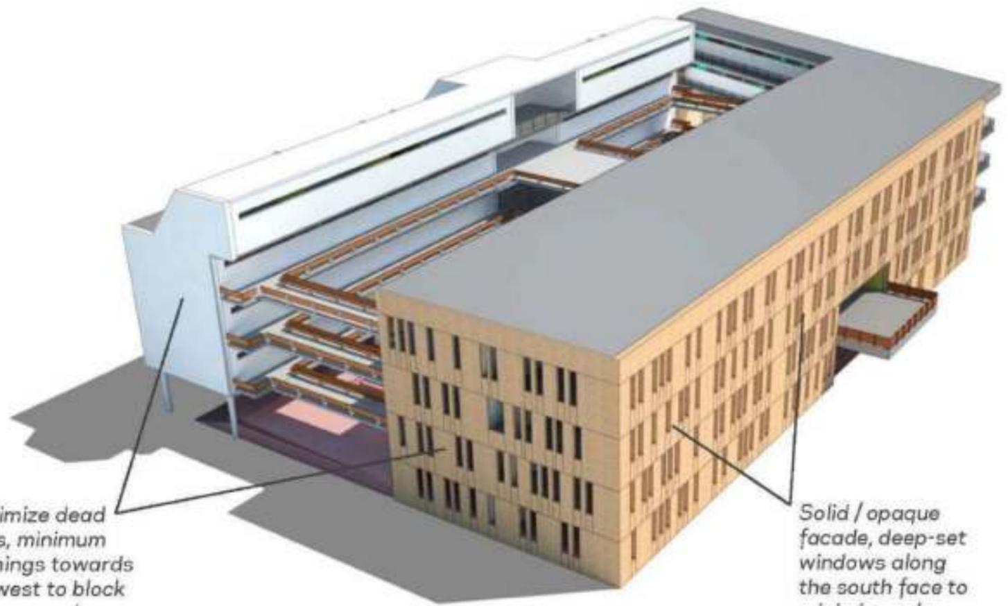
Solid / opaque facade, deep-set windows along the south face to minimize solar exposure
