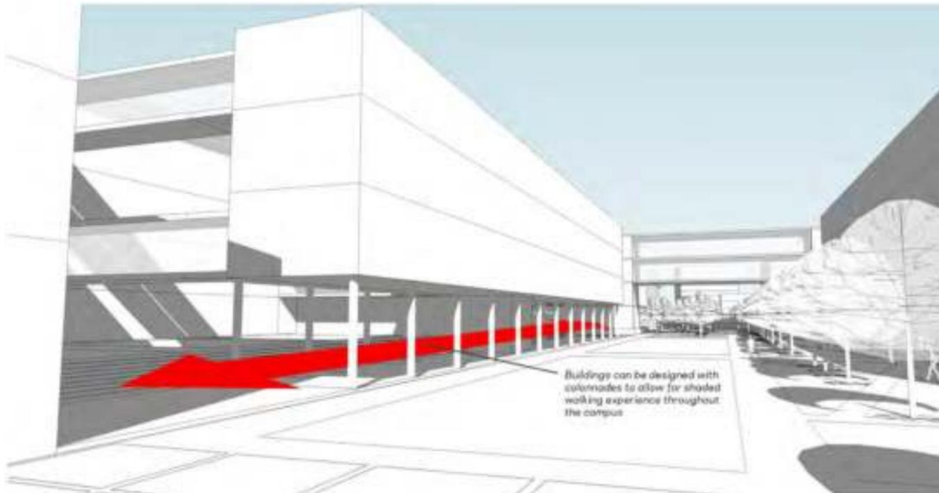
In response to the hot climate of Gurgaon, buildings framing the central quadrangle are lined with colonnades to provide shaded walkways.
