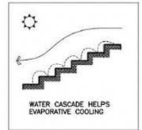
WATER CASCADE HELPS EVAPORATIVE COOLING
