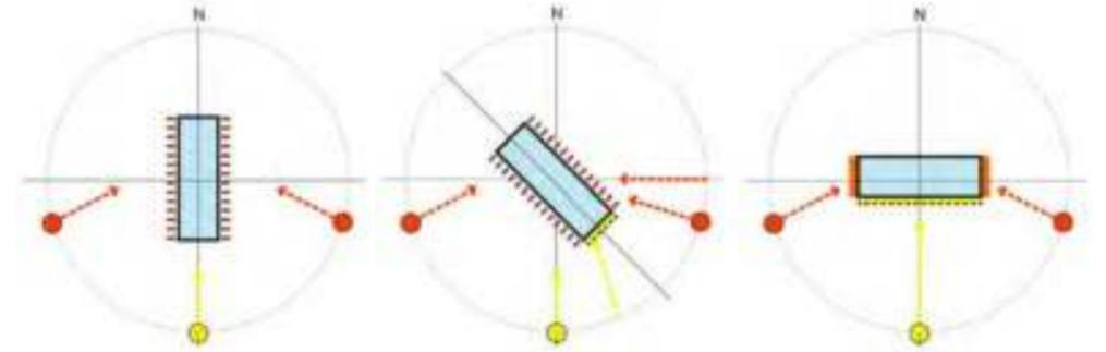
North to south orientation makes controlling solar heat gain extremely difficult
