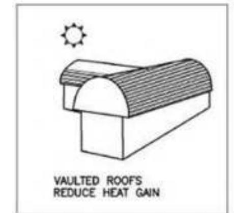
ROOF PROFILE AND OVERHANG: REDUCING HEAT GAIN
